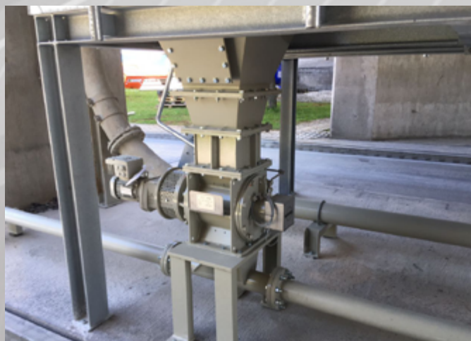
Typical installation of a KREISEL-ceramic rotary feeder
